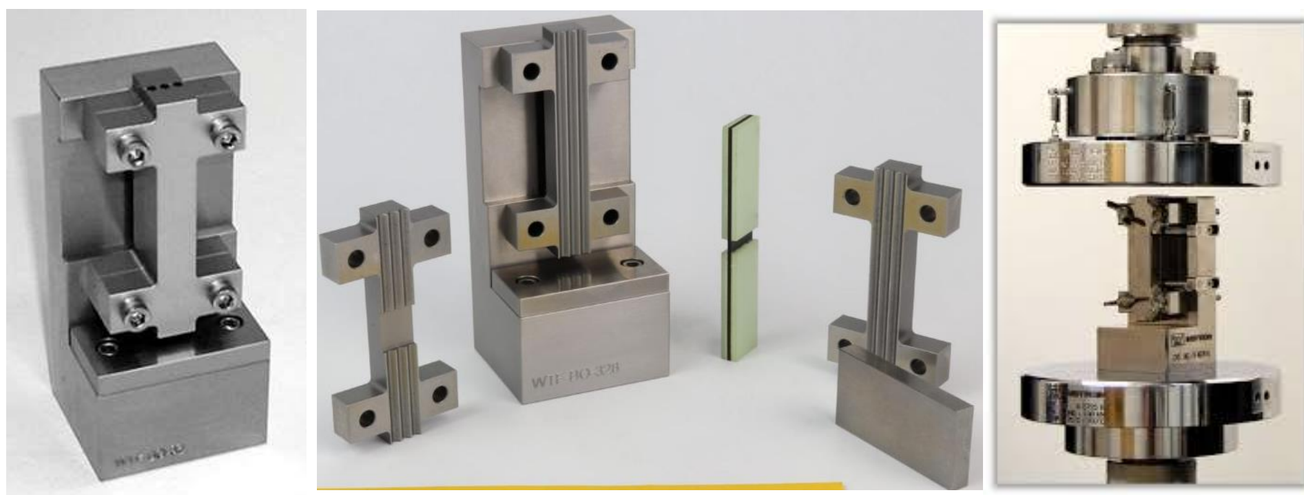
Compression fixture (Modified ASTM D695 Fixture and Base Support)
